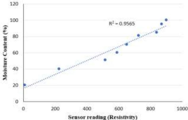
Figure 4. Calibration of soil moisture sensor
