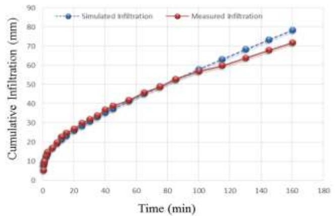
Figure 3. Measured and simulated infiltration graph.
