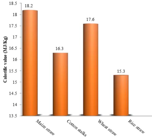
**Figure 8. Calorific values for selected crop residue briquettes.**
