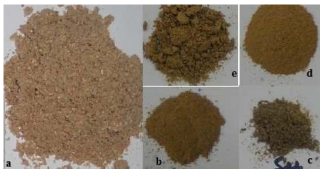
Figure 1. a:corncob before treatment, b:maleic acid treated, c:sulphuric acid treated, d:phosphoric acid treated, e: NaOH treated
